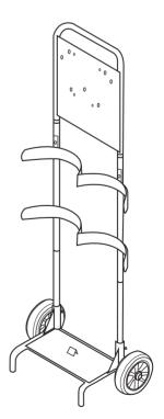
6. Pre-drilled holes in plate for fire alarm installation. Bottom plate for the positioning of a fire bucket.
