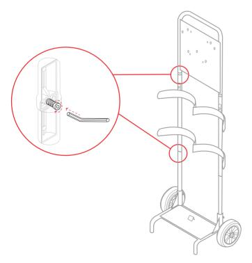
Once all parts are in position, tighten all expanders (A+B) with an allen key to secure the complete frame.
