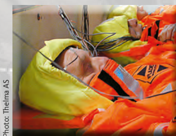
Test pool for thermal testing of immersion suits.
